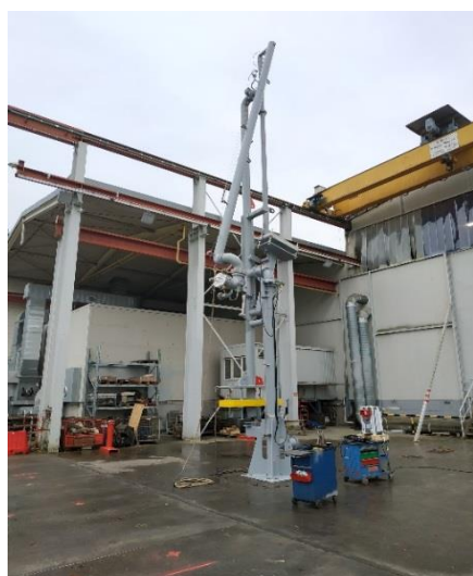
Marine unloading arms at factory premises and unloading at bar Terminal
